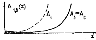
Fig. 18. Abrupt growth of the signal wave far from the boundary, which is due to the effect of superheterodyne amplification.
